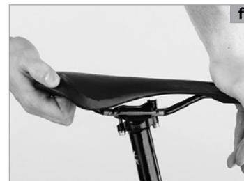
If you have a **single bolt system (a)**, the seat post for most of the sports saddles is designed for a saddle rail diameter of 7 mm. Replacement outer clamps for ovalized saddle rails of 8 mm x 8.5 mm (W x H) as well as for carbon saddle rails bigger than 8 x 8.5 mm are also available. If you are not sure which saddle rail type you have or if you need further information, contact your SCOTT dealer.
