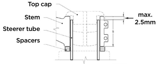
7. Clamp the stem onto the steerer tube with a maximum of 6 Nm **(b)** and respect also the maximum torque value of the stem manufacturer. The lower value indicated on these components has to be accepted as a maximum torque value. Do not overtighten!
