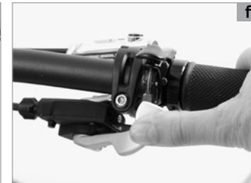
As an alternative, the cable can be retightened directly at the brake in the same way. After readjusting check the functioning and make sure the brake pads do not drag when releasing the brake lever and spinning the wheel (d). Repeated readjustment at the brake lever makes the arm on the brake calliper change its position. This can reduce braking power and result in a complete brake failure in an extreme case. Risk of accident!
