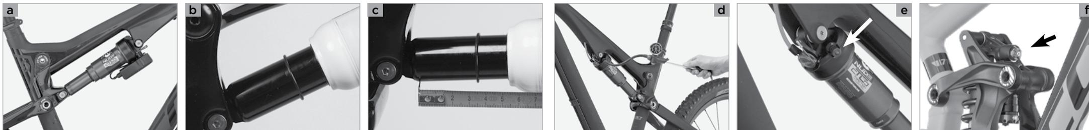
Always make a test ride over different terrains with various surfaces after each change to the setting. Check afterwards the position of the rubber ring/cable tie. Its distance from the wiper is the maximum rear shock travel that you have used.
