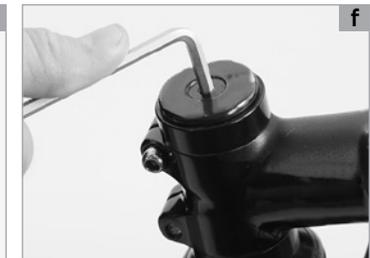
Check after the adjustment or assembly, whether the handlebars are firmly seated in the stem by trying to rotate the handlebars downwards **(a)**. Verify whether the handlebar/stem-combination can be turned relative to the fork. Do this by taking the front wheel between your knees and trying to twist the handlebars. If there is movement, carefully tighten the bolts a little more and check again the proper fit **(b)**.
