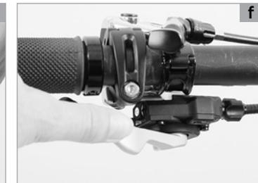
Pulling the small lever located in front of the handlebars from the rider's viewpoint and actuated with the index finger (index finger lever) **(a)** shifts the chain towards the smaller chainwheels/sprockets, i.e. on the right side to the higher gears and on the left side to the lower gears.
