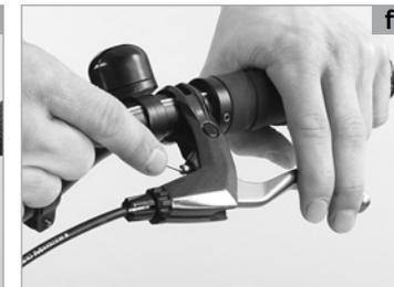
Hydraulic brakes are also fitted with adjusting devices at the brake lever **(a)**. There are different systems. Ask your SCOTT dealer for advice or read the manuals of the component manufacturers on this SCOTT info CD.
