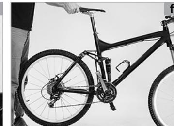
6. Finally, take a good look at the whole SCOTT bike to detect any deformations, colour changes or cracks.
