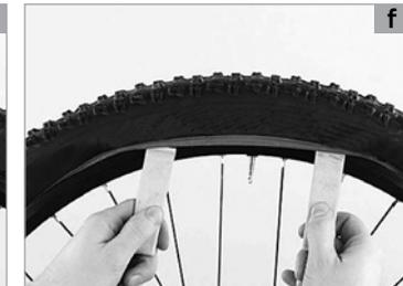
After levering a part of the tyre bead over the edge of the rim you should normally be able to slip off the whole tyre on one side by moving the tyre lever around the whole circumference.
