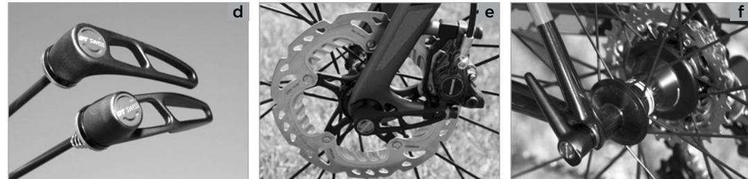
Hold the lock nut on the right side of the hub tight. Turn the RWS quick-release lever clockwise to pre-tighten the RWS system. Depending on the fork mounted or the frame model, the number of turns you need varies. You need at least six, in most cases however more turns. During the first turns you should be able to turn the RWS quick-release lever nearly without resistance.
