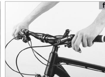
With **disc brakes** you should have a stable pressure point at once. If you have to actuate the brake lever more than once to get a positive braking response, have the SCOTT bike checked by your SCOTT dealer immediately.
